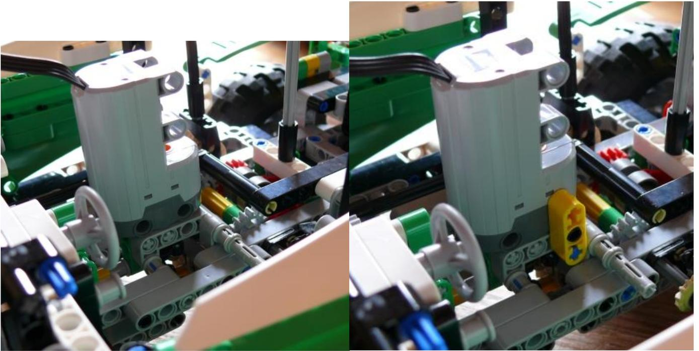
Return the model. Align the front wheels and push the axle thru the knob wheel so it plugs into the servomotor. I used a screwdriver to do this because my fingers are too big.
