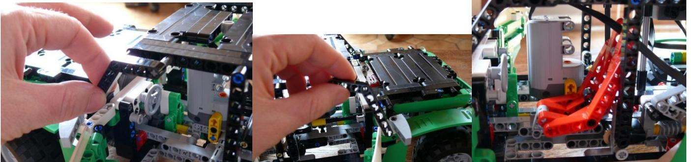
Plug the receiver cable on the battery box, and insert the box into the car. Add a pin to lock the battery box in place.
